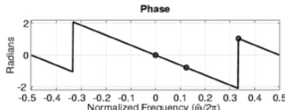
(e) Use Linearity & Frequency response at  $\hat{\omega}=0$ ,  $\hat{\omega}=\pi/4$  and  $\hat{\omega}=2\pi/3$ . These are marked on the plots of the frequency response.
