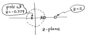
For the second system only the signs on y[n-2] and x[n-2] change, so we can write H(Z) immediately:
