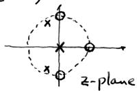
(c) The zeros of the numerator polynomial are on the unit circle at  $Z=e^{j0}$ ,  $Z=e^{j\pi/2}$  and  $Z=e^{j\pi/2}$  when  $x[n]=Ae^{j4}e^{j\hat{\omega}n}$ , the output y[n] is  $y[n]=H(e^{j\hat{\omega}})\cdot Ae^{j4}e^{j\hat{\omega}n}$  There the output will be zero when  $H(e^{j\hat{\omega}})=0$ . That is, for  $\hat{\omega}=0$ ,  $\hat{\omega}=\pi/2$  and  $\hat{\omega}=-\pi/2$ .
