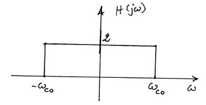
Ideal low-pass filter with gain equal to 2 and  $\omega_m \leq \omega_c \leq 2\omega_c - \omega_m$  (in fact, a non-ideal low-pass filter will also work).
