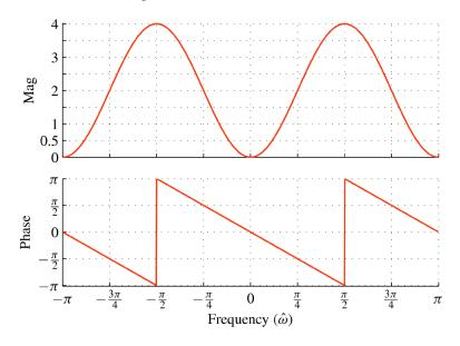
(d) Carefully sketch and label a plot of the principal value of the  $\angle H(e^{j\hat{\omega}})$  for  $-\pi < \hat{\omega} < \pi$ .
