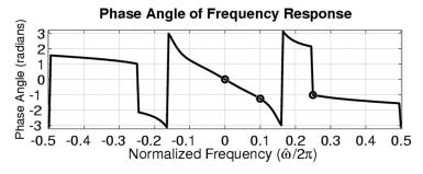
(b) The discontinuity at  $\hat{\omega}=2\pi(0.25)$  is caused by the zero near  $\hat{\omega}=2\pi(0.25)$ . There is a sign change in  $\mathcal{H}(\hat{\omega})$  which means the phase changes by  $\pi$ . The discontinuity at  $\hat{\omega}=2\pi(0.17)$  is a  $2\pi$ -jump" which happens when the principal value of the phase tries to cross  $\pi$ . The arctangent calculation flips the value from  $\pi$  to  $\pi$  creating a " $2\pi$  jump."
