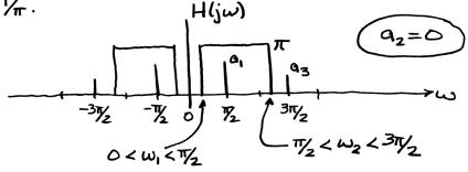
$$H(j\omega) = \begin{cases} 0 & |\omega| < \omega_1 \\ \pi & \omega_1 \le |\omega| \le \omega_2 \\ 0 & \omega_2 \le |\omega| \end{cases}$$
